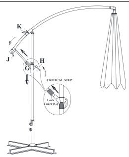
**Step 5:** Slide back the lock cover (G) away from the vertical lift mechanism before lowering the umbrella.
