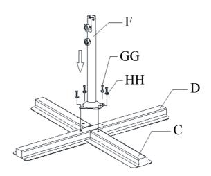
**Step 2:** Attach the holder pole (F) to the cross legs using the bolts (GG) and washers (HH) as shown above. Hand tighten only. Adjust the holder pole (F) to be sure that it is positioned correctly on the base and tighten the bolts. Be Careful to not over tighten the bolts.
