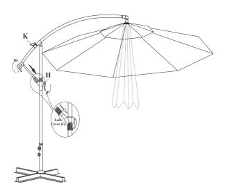
**Step 3:** When the umbrella arm is full extended, lock the two clamps (K and H). Slide the lock cover (G) into the locking mechanism on the back side of the vertical lift mechanism.
