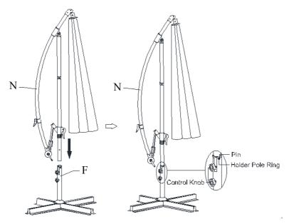
**Step 3:** Insert the main pole of the Umbrella Frame with Canopy (N) into the Holder Pole (F) until the lower fixed stop pin sits on the Holder Pole ring. Tighten the two control knobs to secure the main pole.
