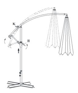
**Step 2:** Unlock the extension arm clamp (K) and the vertical lift mechanism clamp (H). Extend the umbrella extension arm outwards while lifting the vertical lift mechanism upwards. This will fully extend the umbrella.
