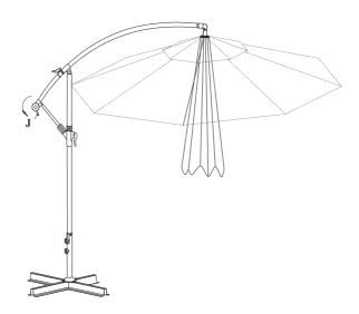
**Step 4:** To open, turn the crank handle (J) clockwise to open the umbrella completely. To close, turn the crank (J) counter-clockwise.
