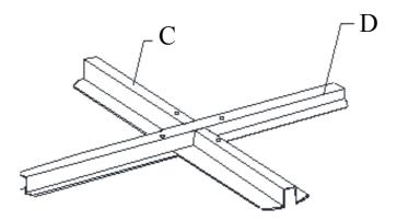
Step 1: Place the upper cross leg (D) on top of the lower cross leg (C).
